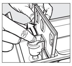
Remove the siphon tube from the compartment & and rinse under warm water.
